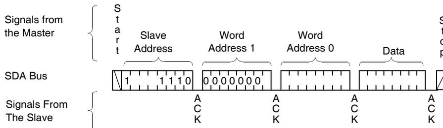
Figure 8. Writing 30 bytes to a 64-byte memory page starting at address 40.
