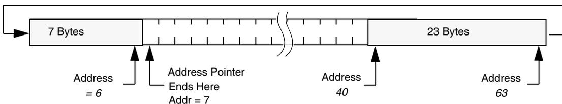
A write to a protected block of memory is ignored, but will still receive an acknowledge. At the end of the write command, the X1226 will not initiate an internal write cycle, and will continue to ACK commands.
