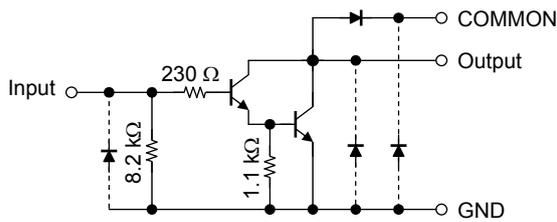
Note: The input and output parasitic diodes cannot be used as clamp diodes.
