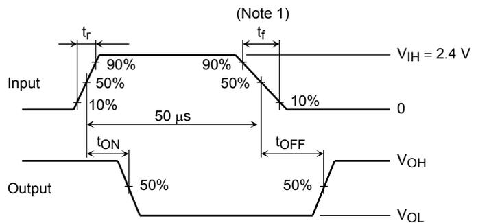
Note 1: Pulse Width 50  $\mu$ s, Duty Cycle 10%
