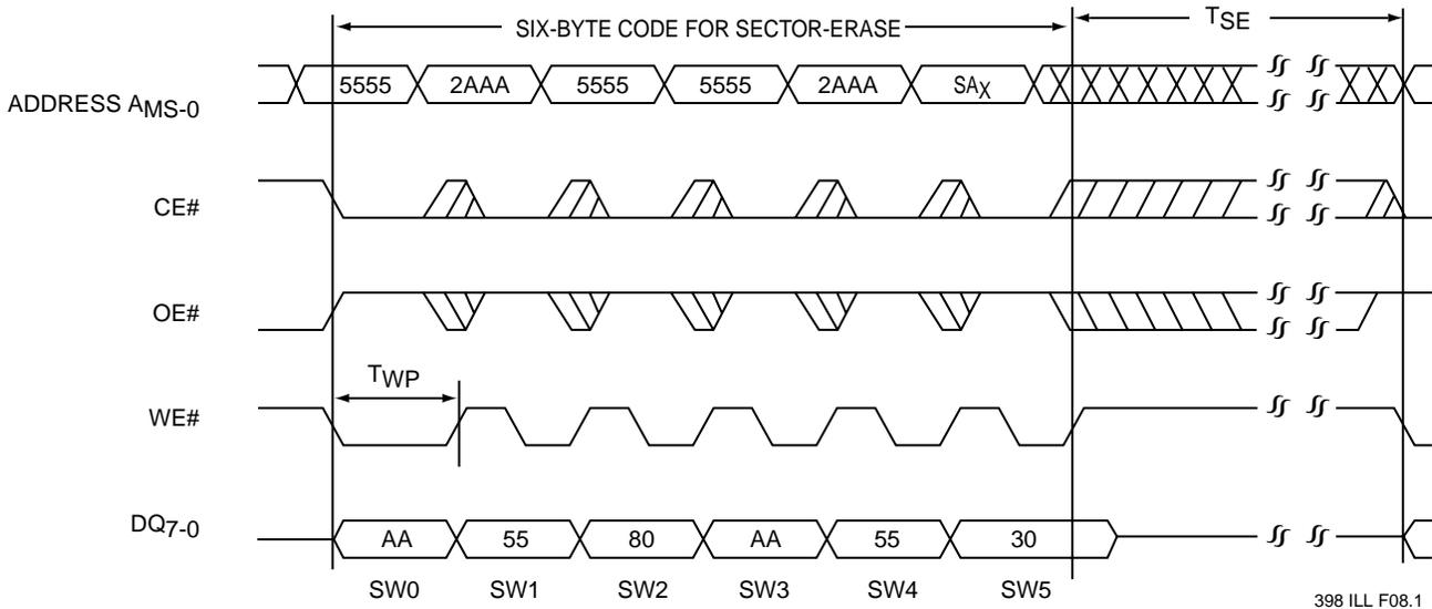
Note: This device also supports CE# controlled Sector-Erase operation. The WE# and CE# signals are interchangeable as long as minimum timings are met. (See Table 10)
