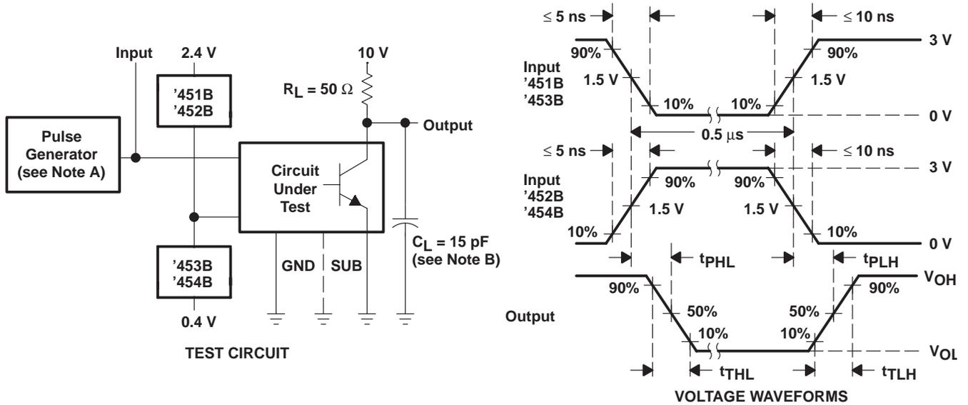
NOTES: A. The pulse generator has the following characteristics: PRR  $\leq$  1 MHz,  $Z_O = 50 \Omega$ .
