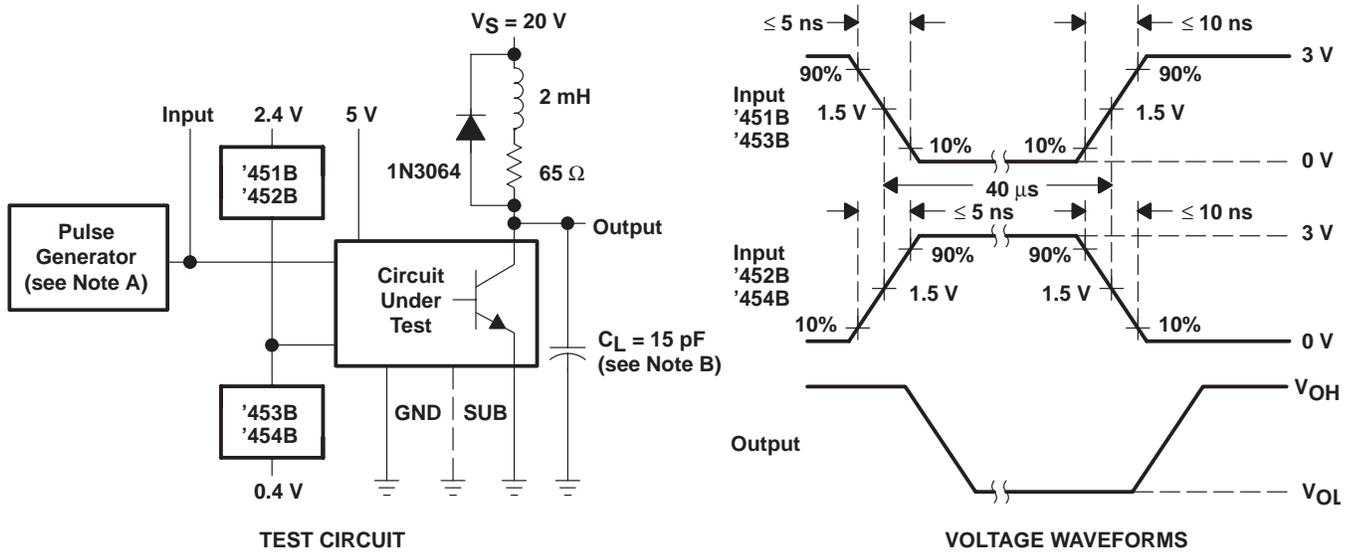
NOTES: A. The pulse generator has the following characteristics: PRR  $\leq$  12.5 kHz,  $Z_O = 50 \Omega$ .
