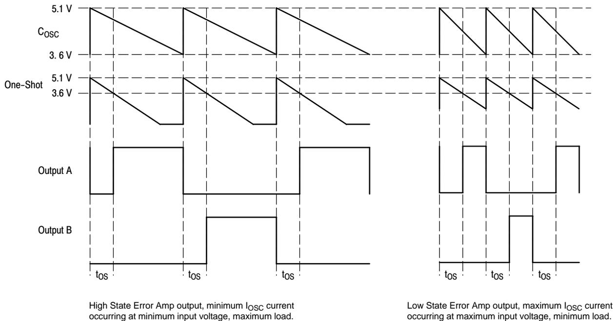
Figure 15. Timing Diagram
