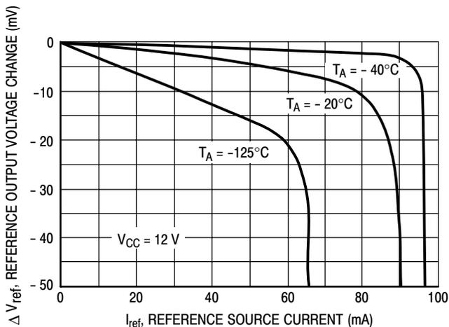
Figure 8. Reference Output Voltage Change versus Source Current
