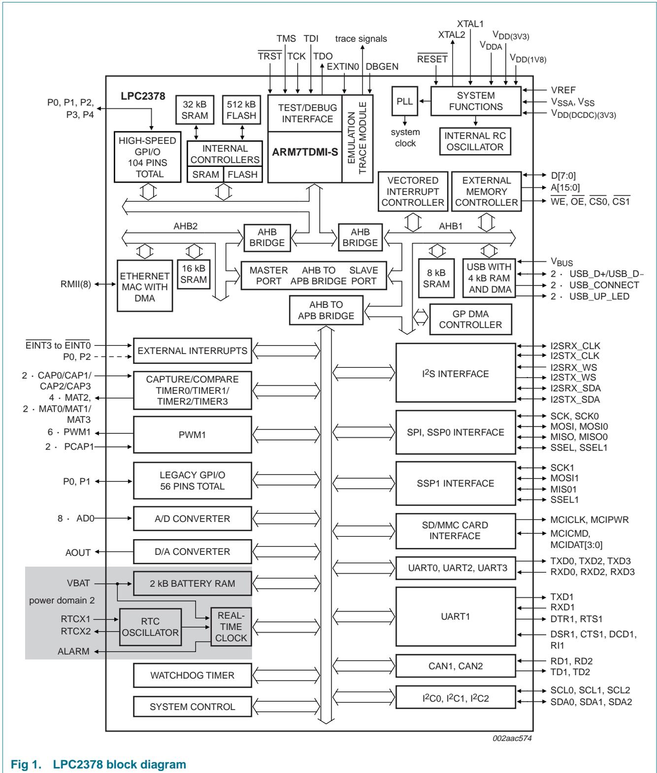
Fig 1. LPC2378 block diagram
