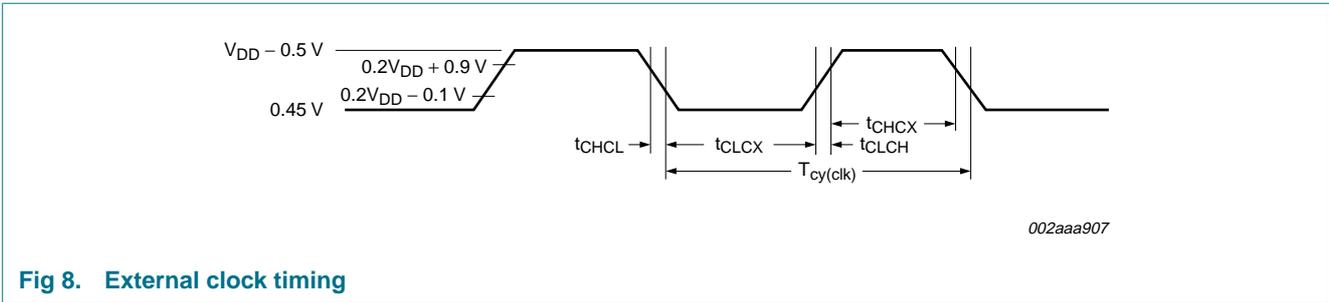
Fig 8. External clock timing
