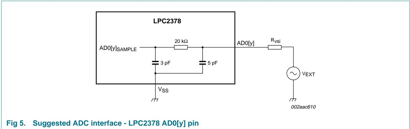
Fig 5. Suggested ADC interface - LPC2378 AD0[y] pin
