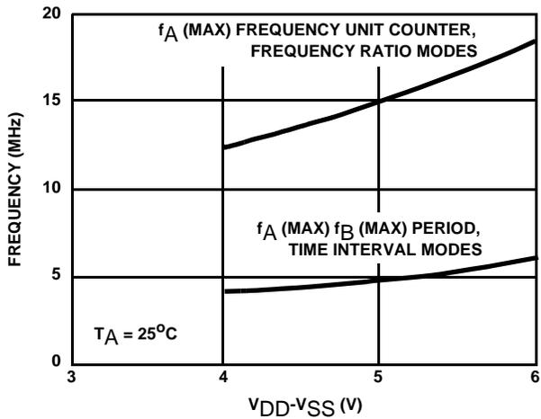
FIGURE 2. f<sub>A</sub>(MAX), f<sub>B</sub>(MAX) AS A FUNCTION OF SUPPLY
