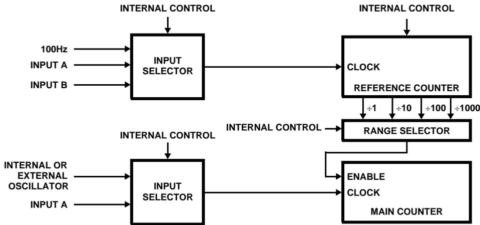
FIGURE 8. SIMPLIFIED BLOCK DIAGRAM OF FUNCTIONS IMPLEMENTATION
