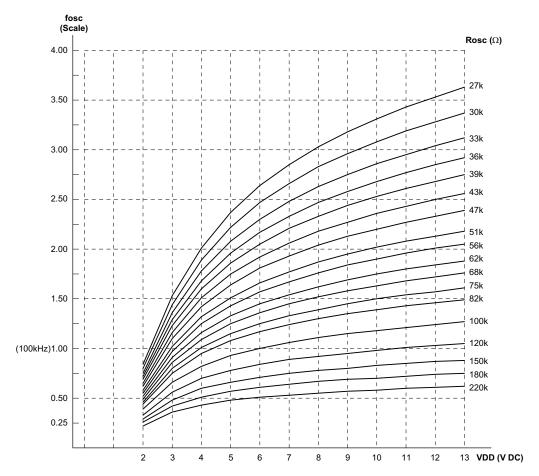
The recommended oscillator frequency is  $f_{OSCD}$  (decoder)  $\cong 50~f_{OSCE}$  (HT12E encoder)  $\cong \frac{1}{3}~f_{OSCE}$  (HT12A encoder).
