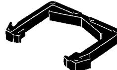
**Note:** P6B-C2 Hold-down Clips cannot be used for G6B-1174P-US.**ALL DIMENSIONS SHOWN ARE IN MILLIMETERS.**
