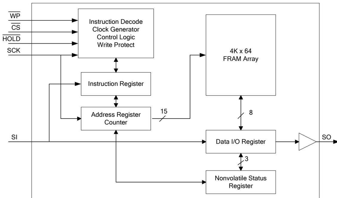
Figure 1. Block Diagram
