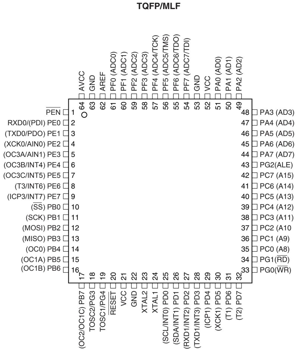
Note: The bottom pad under the QFN/MLF package should be soldered to ground.
