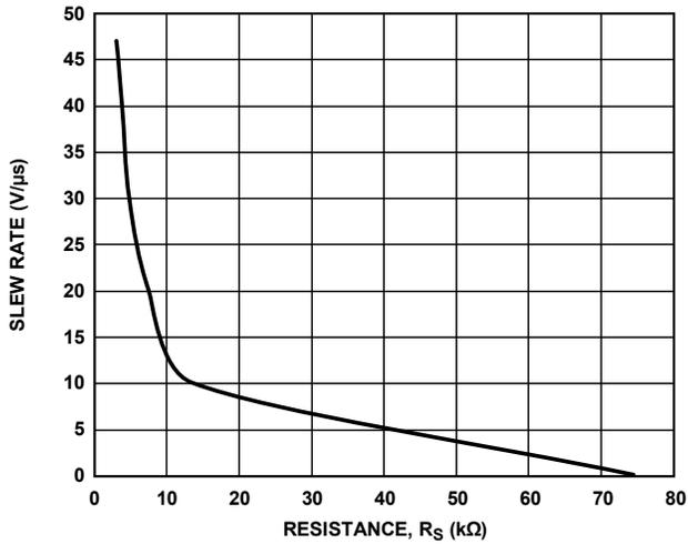
Figure 6. Driver Slew Rate vs. Resistance,  $R_S$
