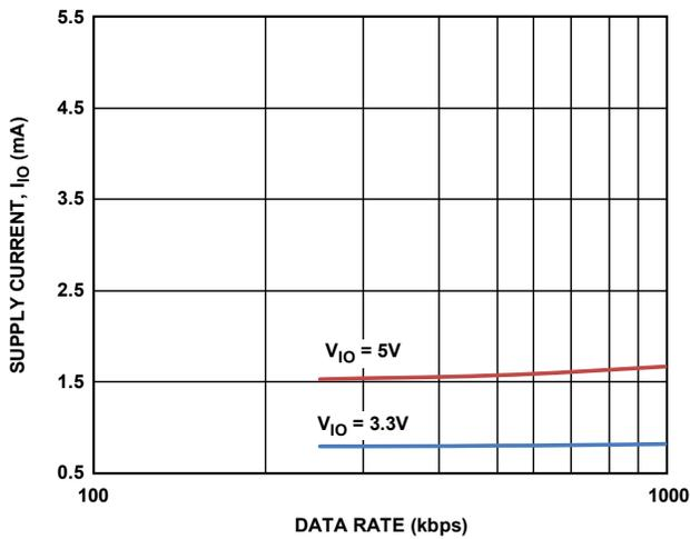
Figure 7. Supply Current,  $I_{IO}$  vs. Data Rate
