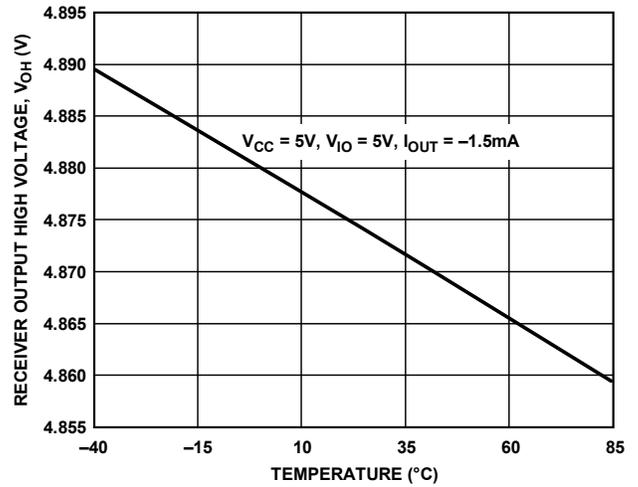
Figure 20. Receiver Output High Voltage vs. Temperature
