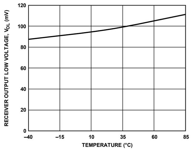
Figure 21. Receiver Output Low Voltage vs. Temperature
