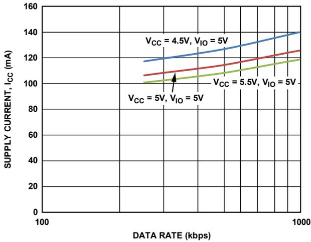
Figure 5. Supply Current,  $I_{CC}$  vs. Data Rate
