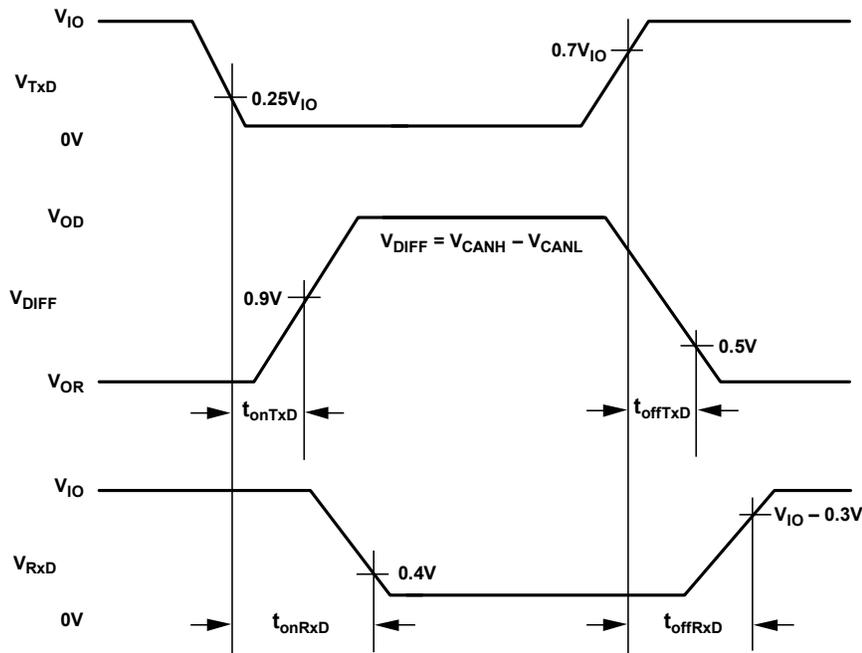
Figure 2. Driver Propagation Delay, Rise/Fall Timing
