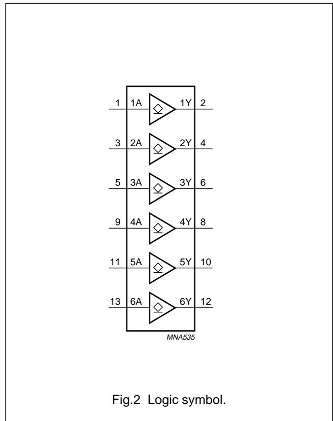
Hex buffer with open-drain outputs
