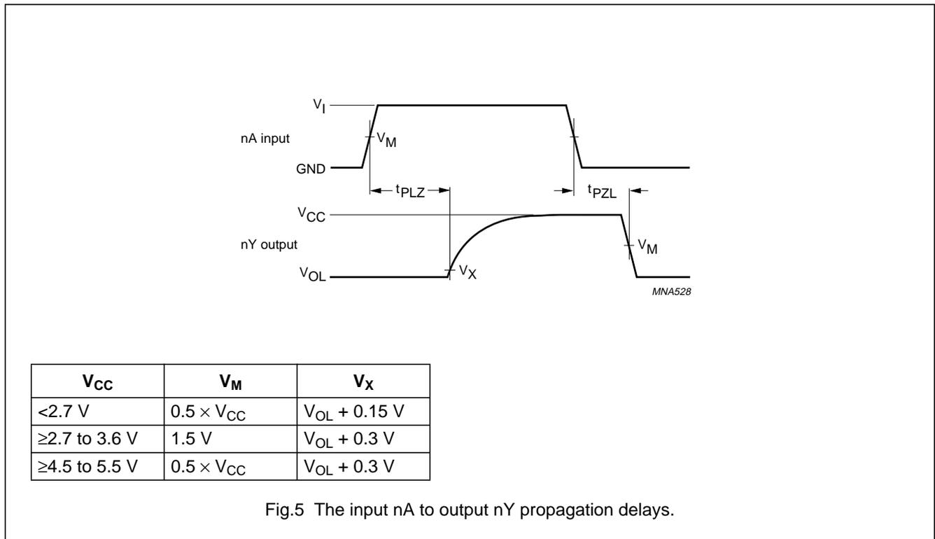
Hex buffer with open-drain outputs
