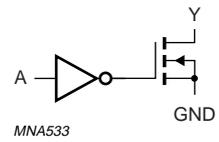
Fig.4 Logic diagram (one gate).
