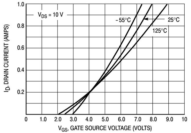
Figure 2. Transfer Characteristics
