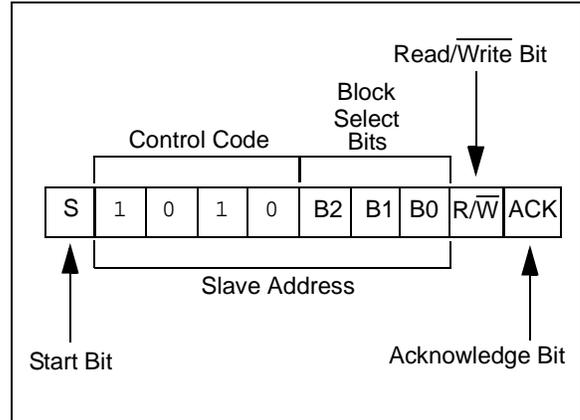
**FIGURE 5-2: ADDRESS SEQUENCE BIT ASSIGNMENTS**
